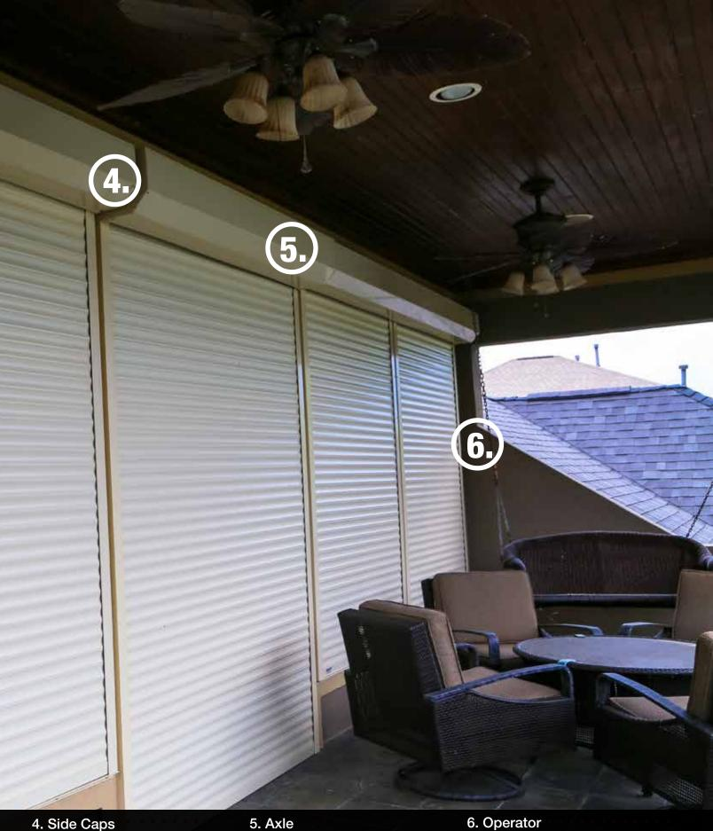
**4. Side Caps** Heavy duty aluminum end caps connect the housing to the rails. They support the weight of the axle and shutter curtain. **5. Axle** The axle is the interior rolling mechanism that the shutter curtain rolls upon. Larger shutter systems require a large axle to prevent sagging across wider lengths. **6. Operator** Available in manual and motorized operation. Manual operators for smaller shutter systems, and motorization for easy push button operation as well as automation.
